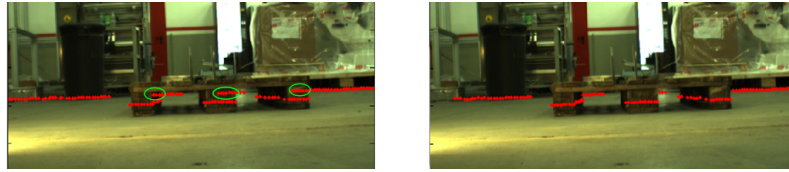
Figure 4.8: Laser points over the image, filtering effect
