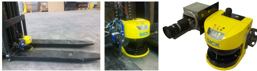
(a) Devices mounted on an experimental AGV (b) Prototype version (c) Final configuration of the sensors
