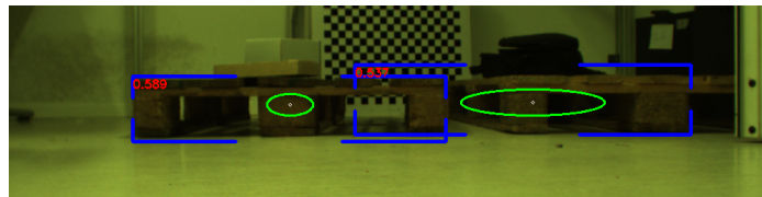
Figure 3.33: Identification failure: covariance dimensions
