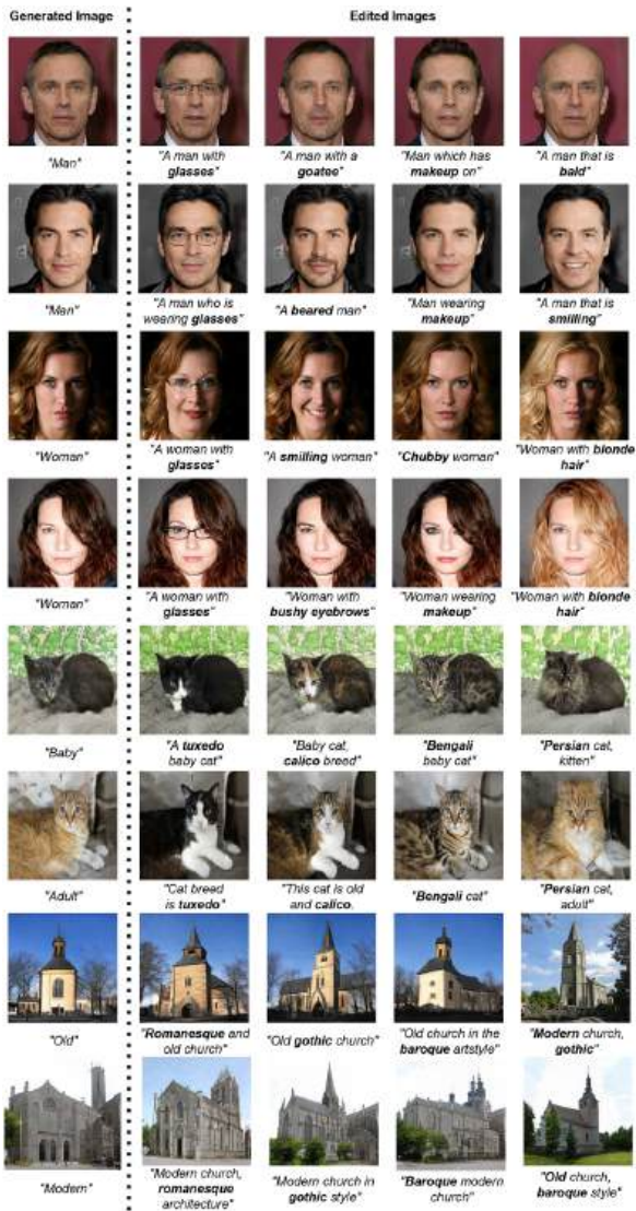
Fig. 1. Examples of generated and edited images. On the right side, the generated images use the class conditioning generation of StyleGAN in order to get a base image. The remaining images represent the edited ones, obtained using the given text prompt mentioned below each image. We used bold to highlight the requested feature.
