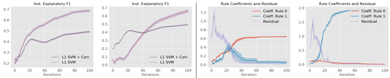
Figure 2: Explanatory feedback (+ Corr.) can drive an active L_1 SVM towards the right concept (colors problem). (Left) instantaneous F_1 score of the LIME explanations for rule 0 (leftmost) and rule 1 (left middle). (Right) Decomposition of the learned weight vector when the corrections push toward rule 0 (right middle) and rule 1 (rightmost). (Best viewed in color)
