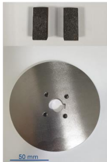
Fig.5.2: samples used at the sub-scale dynamometer: coupons of friction materials and disc.
