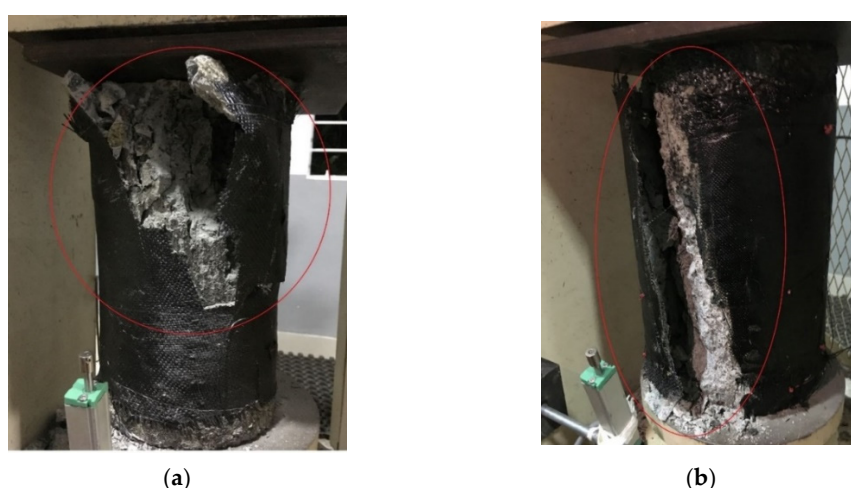
Figure 9. Failure pattern of confined HSBFRP specimen exposed to elevated temperature: (a) C-E0C2S2B400; and (b) C-E1C2S2B400.
