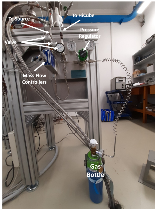
Figure 6.5: The system used to inject a specific quantity of noble gas on the front face of the source and on the conical surface in front of it. The gas flux, from the gas bottle, is regulated by the Mass Flow Controller and the pressure regulator.
