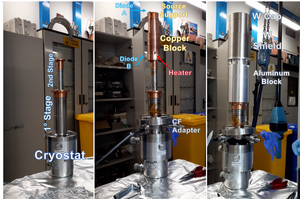
Figure 6.3: Photos of the cryocooler of the PsICO apparatus. The two-stage commercial cryocooler Sumitomo CH-204S-N (left), the copper block and source support mounted on the second stage with elements to control the moderator temperature (middle), and the aluminum block and tungsten elements mounted on the first stage (right).
