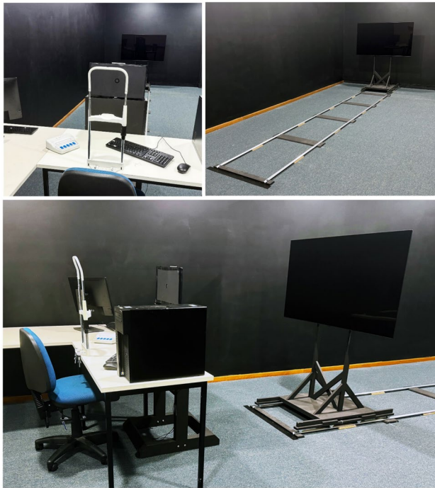
Fig. 1 The image shows the apparatus set up in the testing area from different angles (overhead lights are on for visibility, during testing the ambient lighting was dimmer and illuminated by a lamp). The nearby walls were blacked out
