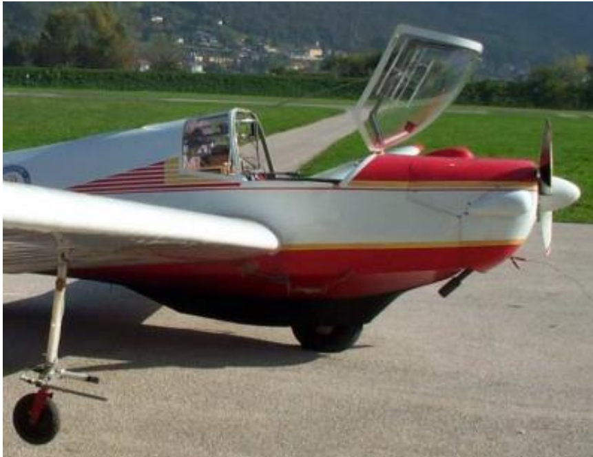
Figure 3.1. The Scheibe Falck SF 25C. Notice temperature and humidity sensors mounted on the left-side leg of the motorglider undercarriage (lower-right corner of the picture). Picture by courtesy of Massimiliano de Franceschi.
