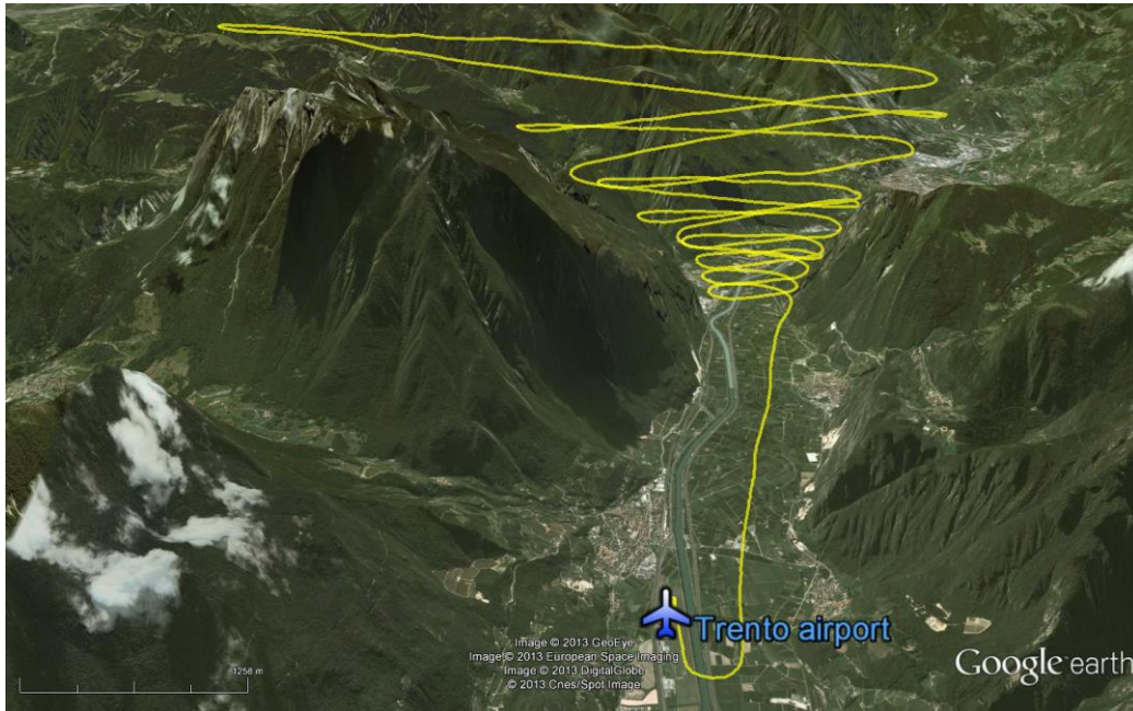
Figure 4.1. 3D representation of flight #N trajectory exploring the target Adige Valley cross section. View is from N. Image © Google Earth, © 2013 GeoEye, © 2013 European Space Imaging, © 2013 DigitalGlobe, © 2013 Cnes/Spot Image.
