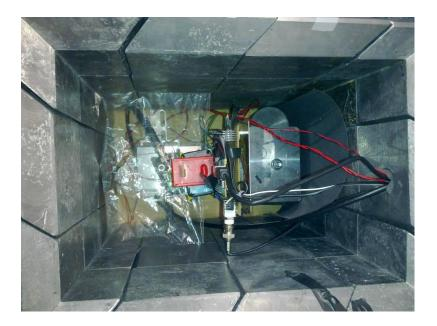
Figure 4.6: Experimental setup used for the experiments with  $\gamma$ -ray sources. It can be noticed the position of the sources that are contained in the red and blue boxes. Two different sources (low activity <sup>133</sup>Ba and <sup>22</sup>Na) have been used to reach a number of events well discernable from the background radiation activity. The sources are positioned as close as possible to the crystal.
