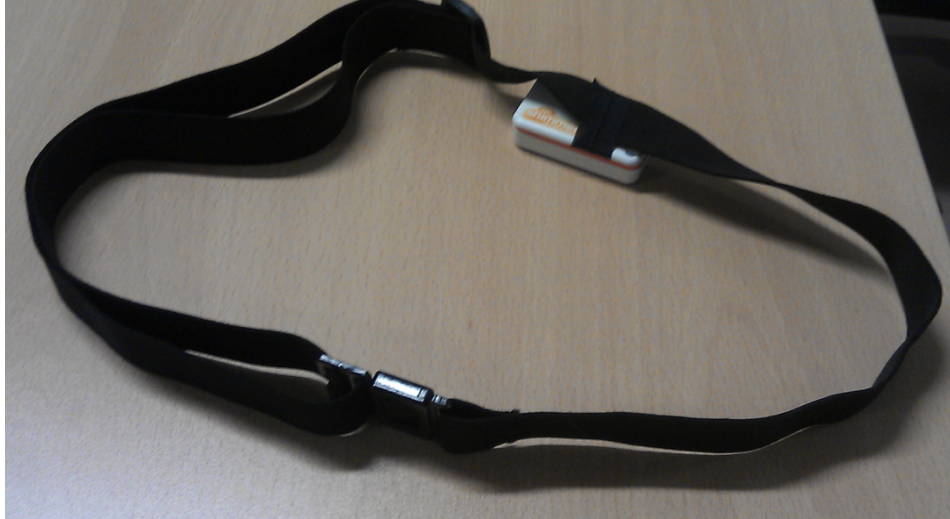
Figure 5.5: Shimmer accelerometer on the elastic band
