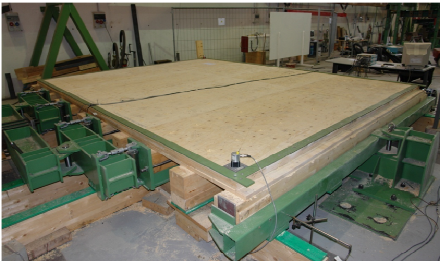
Fig. 76 Floor reinforced with plywood panels
