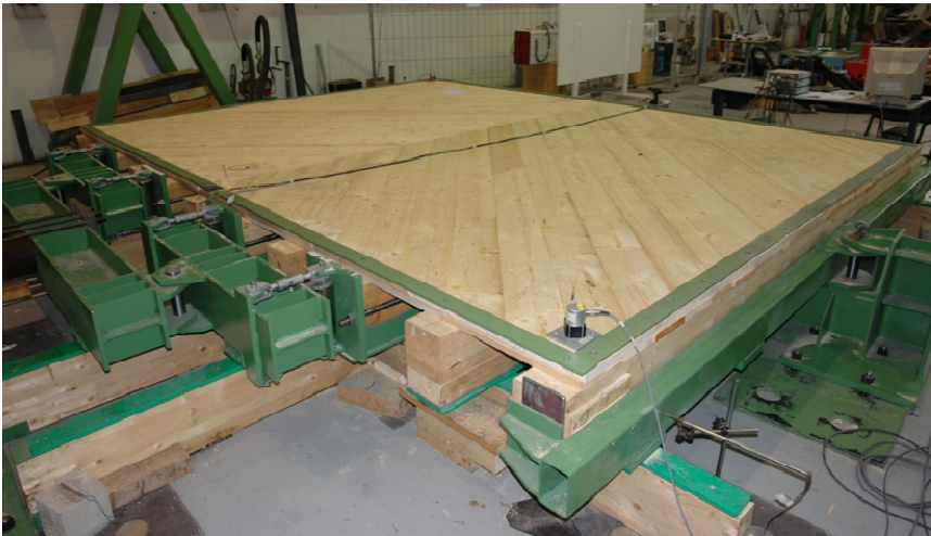
Fig. 6 Floor reinforced with timber boards
