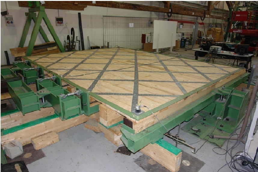
Fig. 56 Floor reinforced with steel plates
