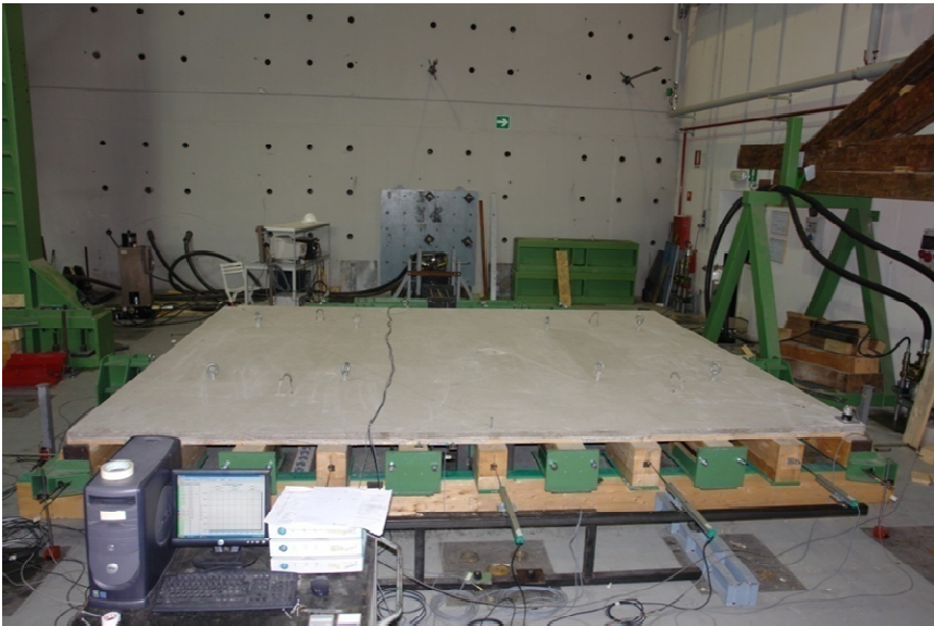
Fig. 10 Floor with concrete slabs above existing boards
