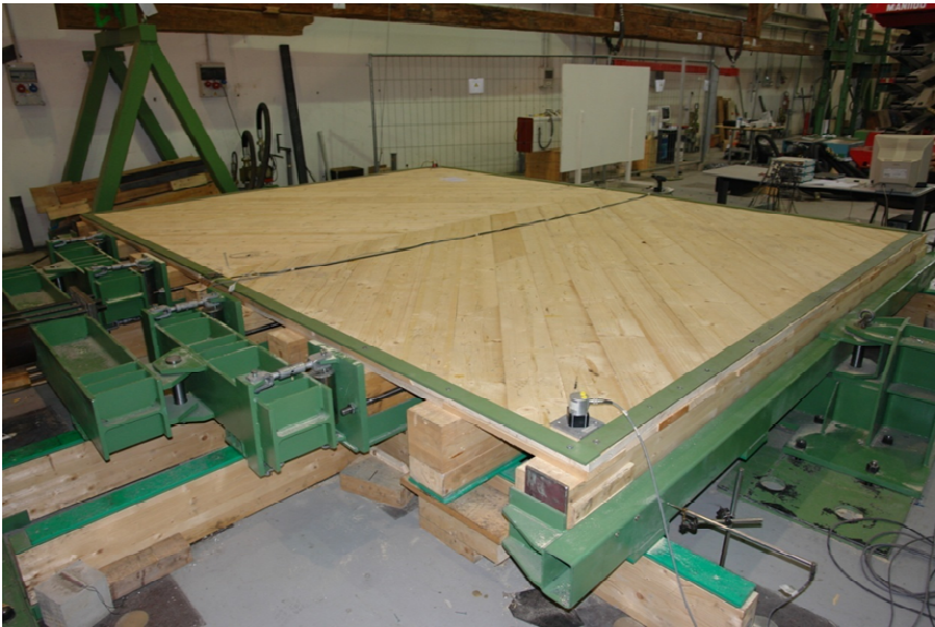
Fig. 46 Floor reinforced with timber boards
