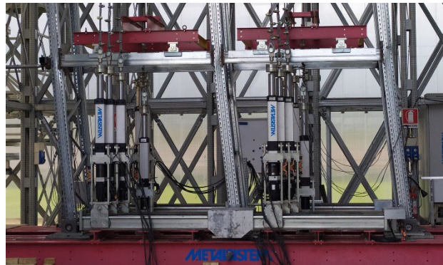
Figure 3. View of the vertical loading equipment mounted on the rails and of the loads transfer system.
