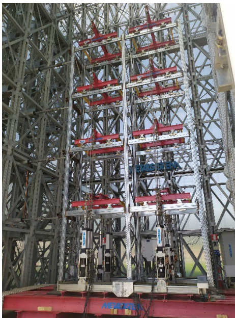
Figure 2. Specimen in the testing rig, with four horizontal actuators and fourteen vertical actuators.
