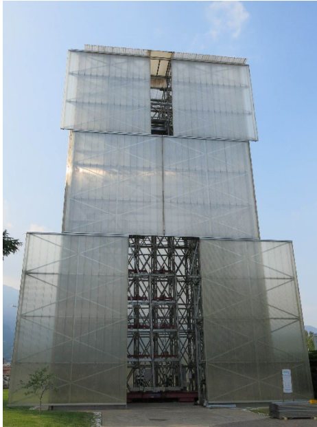
Figure 1. The testing tower and a specimen built-in.
