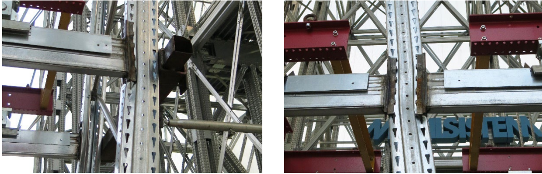
Figure 12. Details of the plastic deformations of the first level joints for a test performed with Q = 1/3 ESL.
