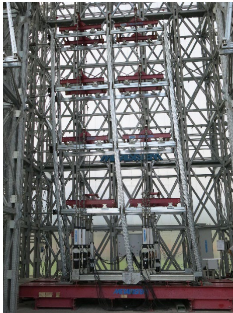
Figure 13. Collapse of a full-scale rack subjected to push-over loading with Q = 1/3 ESL.
