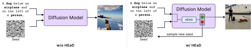
Figure 3.1: Overview of the HEaD pipeline: during the generation process, HEaD assesses whether all designated objects will be accurately represented in the final image, determining if the generation process should continue or be restarted with a different seed.
