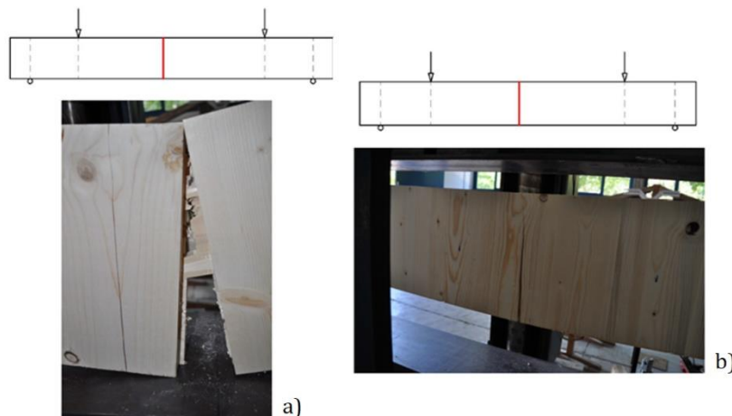
Figure 13: failure mode in long beams, B 02 (specimen #2),a, and B 01 (specimen #3),b.
