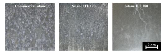
Figure 2.28 Appeareance of the samples after 72 hours of exposure in the salt spray chamber
