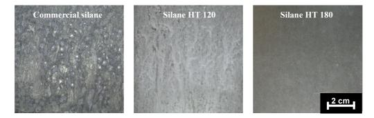
Figure 2.27 Appeareance of the samples after 24 hours of exposure in the salt spray chamber
