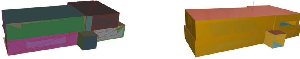
Fig. 74. House 01: (a) FEM based representation generated from the parser transformer writer; (b) corresponding gbXML model derived from the graph structured Digital Twin and validated through FME.
