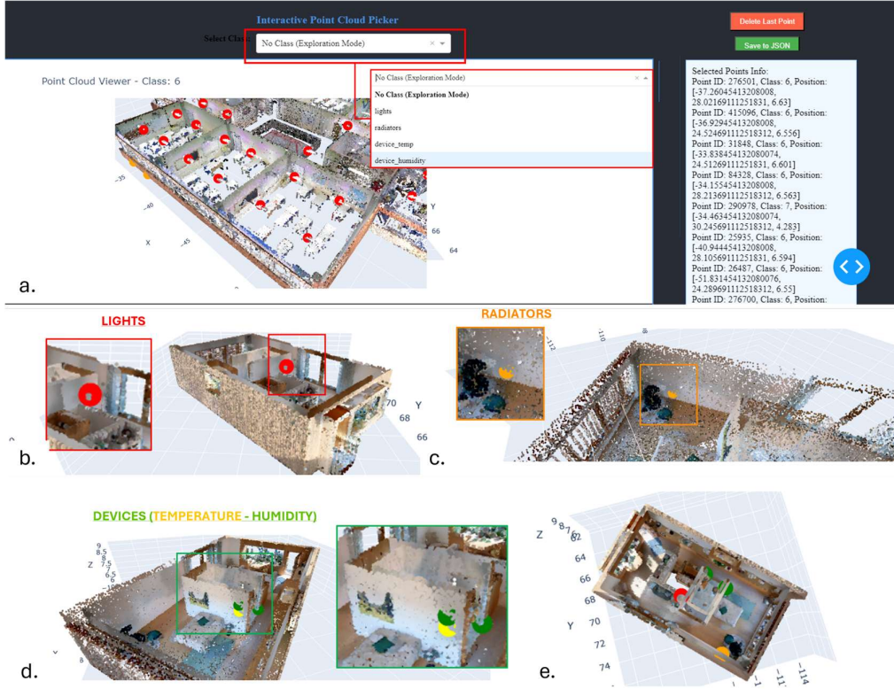
Fig. 34. Results of the developed tool for manual detection and classification of energy-related elements. (a) User interface with lighting elements highlighted, (b) detected lights, (c) detected radiators, (d) detected devices and sensors, and (e) top view of the scene after element detection.
