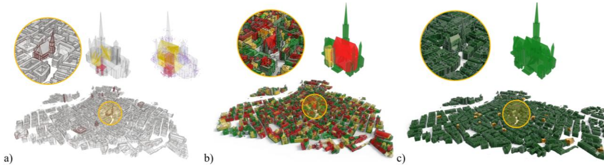
Fig. 99. First outputs of city level application: the graph structure here is used for repairing LoD2 building models from a topologic point of view.
