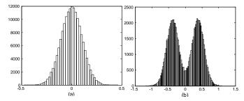
Fig. 4: Noise distribution (real part) after the FFT demodulator, 3bit PCM,  $\sigma_{IN}$ /FS=0.1 (a) and  $\sigma_{IN}$ /FS=1 (b), obtained from a record of 50 OFDM symbols, made of 2048 samples each. The error samples have been normalized to the QAM symbol amplitude. The imaginary noise component shows the same distribution.
