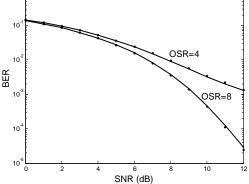
Fig. 6: Sigma-Delta dynamic range optimized to input signal power. The continuous line represents the analytic model (3), while the dots represent simulation results.
