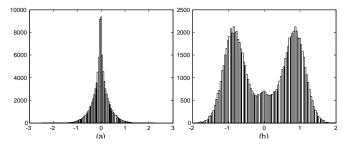
Fig. 7: Noise distribution (real part) after the FFT demodulator, single-bit Sigma-Delta,  $\sigma_{IN}/FS=0.1$  (a) and  $\sigma_{IN}/FS=1$  (b), obtained from a record of 50 OFDM symbols, made of 2048 samples each. The error samples have been normalized to the QAM symbol amplitude. The imaginary noise component shows the same distributions.
