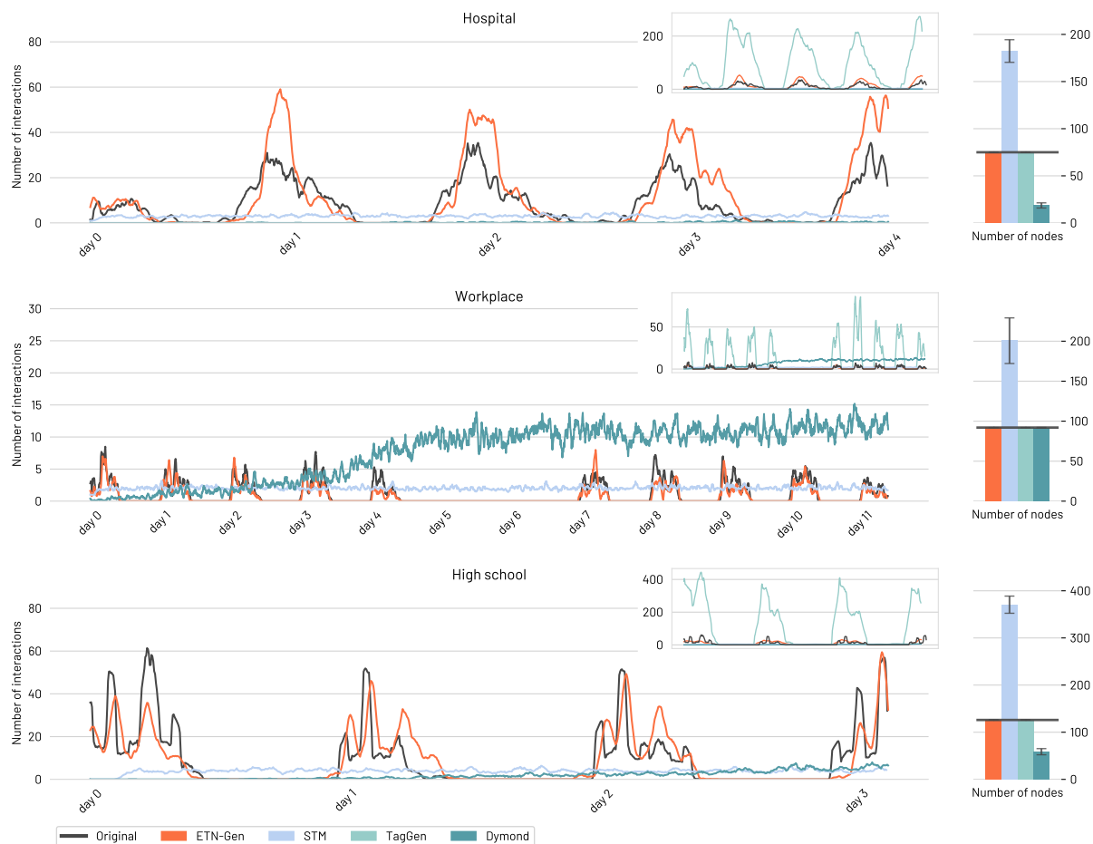
Figure 5.2: Number of interactions in the generated network vs. competitors. Number of interactions at each timestamp, each color represents a different generation algorithm, while the original graph is depicted in black. TagGen produces a number of interactions ten times the order of the original network and it only appears in the insets for visibility.
