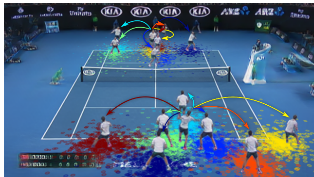
Figure 3.7: Action space learned by our method on the Tennis dataset. Each color represents a learned action and each arrow shows the effects of applying the respective action six times to the initial player. The overlay on the floor shows the distribution of possible ending positions after the application of each action.
