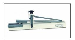
Figure 3.7 Crockmeter test [33].
