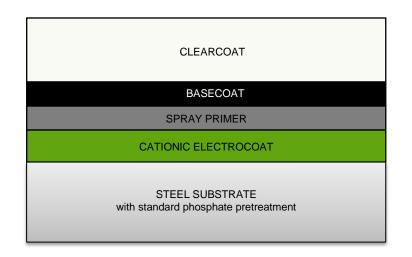
Figure 3.13 The four-layers coating system.
