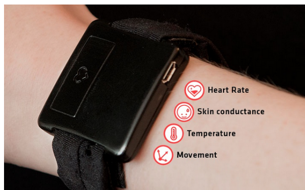
Figure 4.2: Empatica E3 wristband - wearable, lightweight, wireless, multi-sensory data acquisition device
