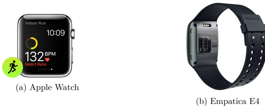
Figure 2.8: Wearable Devices can keep track of physiological signals. The Apple watch can measure activity and heart rate. The Empatica E4 can measure heart rate, electrodermal activity, and skin temperature.
