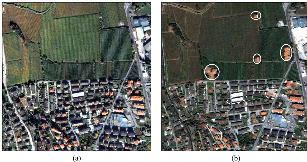
Figure 2.3. Example of change detection problem in VHR optical images. True colour composition of QuickBird pansharpened images acquired in: (a) October 2005, and (b) July 2006. The area of interest is a sub-urban area located close to Trento (Italy). Changes are mainly associated to buildings (see white circles in the right image).
