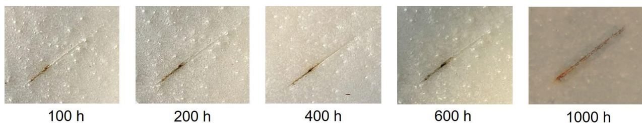
Figure 9. Visual appearance of the scribes during 1000 h of continuous immersion in 0.1M NaCl.
