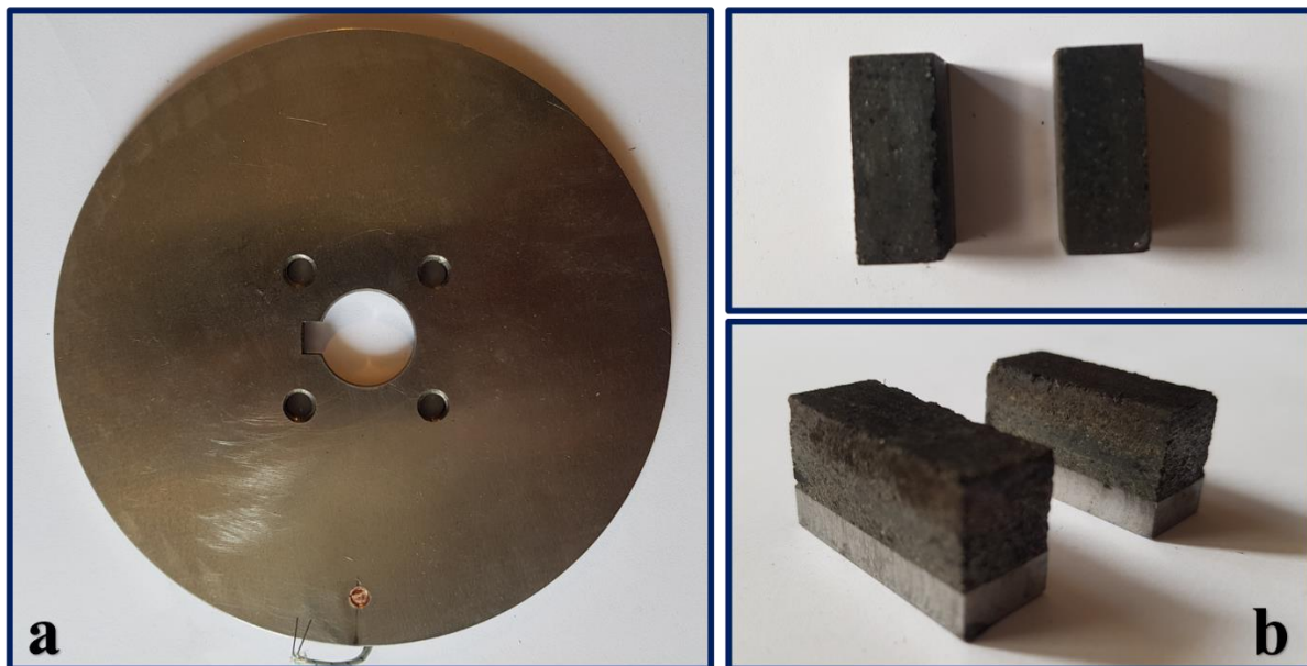
Figure 3-5. Minidyno main components; a: Brake disc, b: Brake pads
