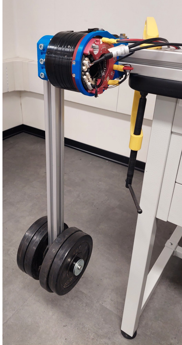
Figure 5.8: Leon's customised actuator on the test bench. The actuator is configured as a hip-roll joint, i.e. with the electronics positioned on its back. It is mounted through FFF-fabricated components on an aluminium profile extrusion, which is clamped on the desk. Another aluminium extrusion, mounted through a FFF-fabricated output flange, acts as link, and gym weights (up to 8 kg) can be positioned at any distance from the rotation axis (up to 0.5 m).
