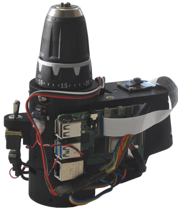
Figure 4.31: The frame of Smart Drill, housing all functional components.
