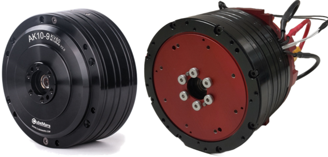
Figure 4.3: On the left, the COTS QDD actuator. On the right, the actuator modified for Leon. Reproduced with permission from Springer Nature. First published in Springer Proceedings in Advanced Robotics, vol 32, pp 58–63, 2025 by Springer Nature [120].
