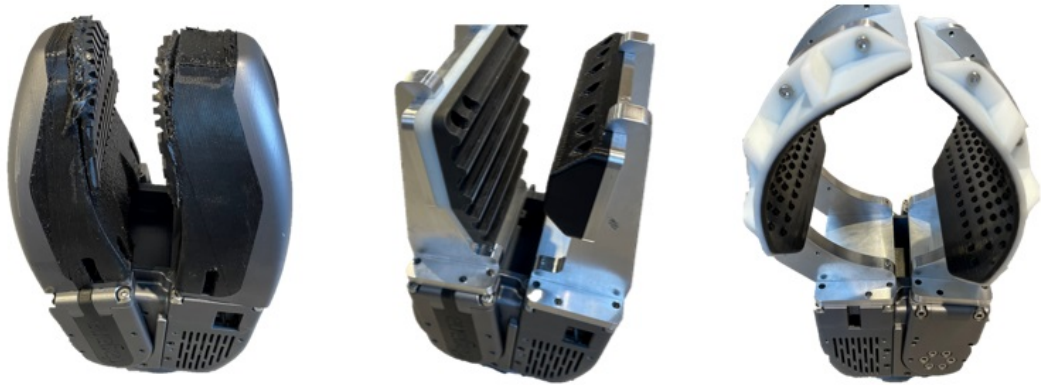
Figure 4.25: Three different grasping modules developed for the DAGANA gripper. On the left, the standard jaws, in the centre, jaws for manipulating planar formwork, and on the right, jaws for grasping tubes. Reproduced with permission from IEEE. First published in [125]. © 2024 IEEE.
