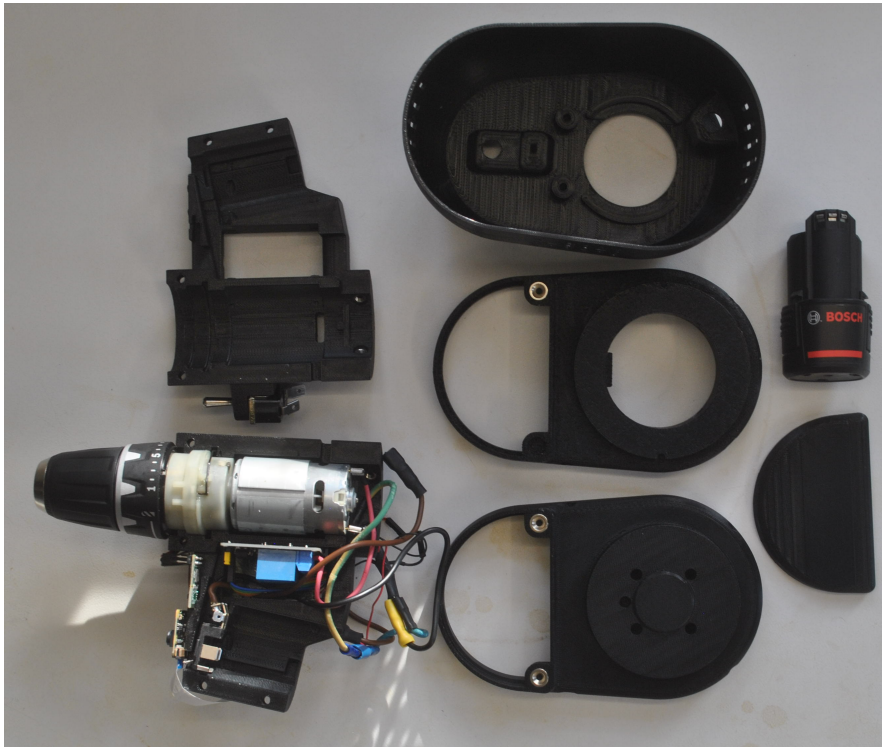
Figure 4.30: Smart Drill, partially disassembled. On the left, the two semi-shell structures of the frame. In the top-middle, the front cover. In the centre and bottom-middle, the couplings. On the right, the battery and its cover.
