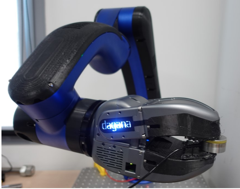
Figure 5.14: The DAGANA gripper pinching a FT sensor on a lightweight robotic manipulator developed by IIT [130]. Reproduced with permission from IEEE. First published in [125]. © 2024 IEEE.
