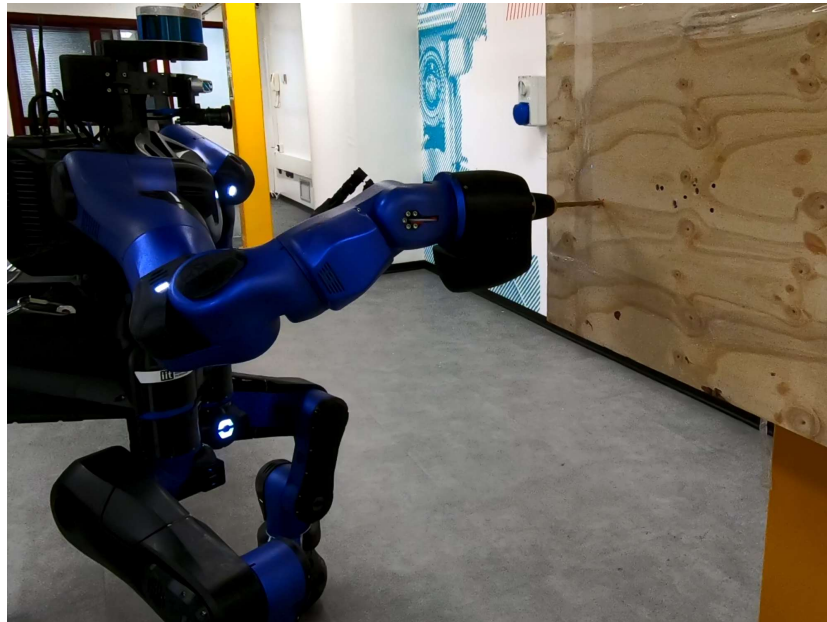
Figure 5.23: The IIT CENTAURO NEXUS [43] drilling a plywood panel with Smart Drill. Reproduced with permission from IEEE. First published in [128]. © 2024 IEEE.
