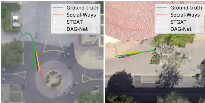
Figure 3.11: Qualitative samples that compare DAG-Net and state-of-the-art methods on Stanford Drone Dataset.
