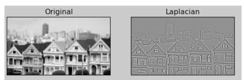
**Figure 17** The potential  $\phi$  represented as the levels of gray of a b/w image (left) and the corresponding Laplacian as calculated by a standard finite-difference method (right).
