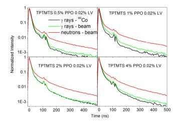
Figure IV. 13. Average pulse shapes for TPTMTS at different PPO concentrations. Each graph shows the comparison between neutrons and gamma rays produced by two different sources.
