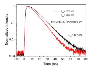
Figure IV. 7. Fluorescence decay for a sample with 4% PPO excited at 280 nm and at 375 nm.
