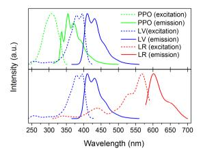
Figure II. 12. Overlap between the different dyes emission and excitation spectra.
