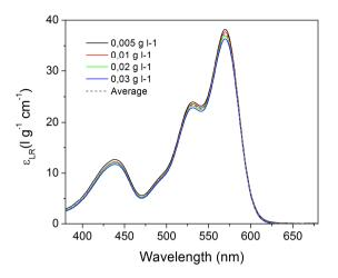
Figure VI. 7. Mass absorptivity as calculated from normalization of measured absorption over concentration.
