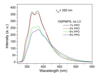
Figure V. 2. Non-normalized fluorescence emission spectra of polysiloxane samples at different PPO concentrations without LV, recorded with 250 nm excitation.
