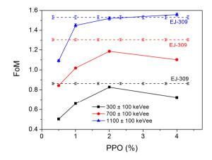
Figure IV. 19. FoM as a function of PPO concentration for TPTMTS with 0.02% LV, at three different energies. FoM of EJ-309 is also shown for comparison.
