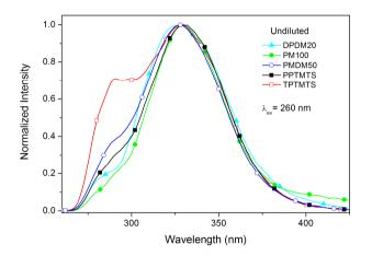
Figure III. 8. Emission spectra of undiluted polysiloxane liquids excited at 260 nm.
