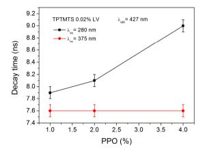
Figure IV. 5. Fluorescence decay time as a function of PPO concentration at the two different excitation wavelengths.
