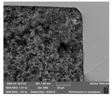
Figure VII. 4. SEM image of the cross-section of a 3D diode filled with 6LiF powder.
