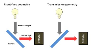
Figure II. 13. Schematic representation of the front-face and transmission geometry employed in the fluorescence measurements of solid samples.
