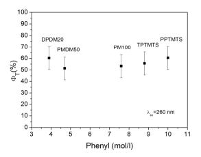
Figure III. 13. Estimation for non-radiative energy transfer efficiency.
