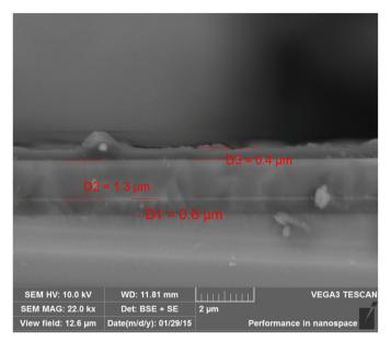
Figure VII. 6. Cross sectional SEM image of a <sup>10</sup>B thin layer deposited on the planar detector surface. 1.3 µm metal layer and 0.6 µm oxide layer are also clearly distinguished.
