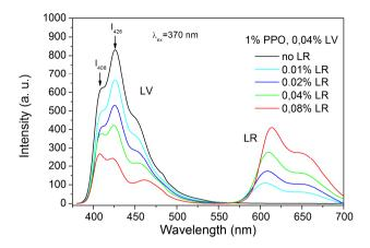
Figure VI. 3. Emission spectra of different samples at fixed 1% PPO and 0.04% LV concentration and with variable amount of LR. Excitation wavelength was fixed at 370 nm.
