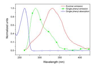
Figure II. 1. Comparison between absorption spectrum, single phenyl emission and excimer emission for phenyl substituted polysiloxane materials.
