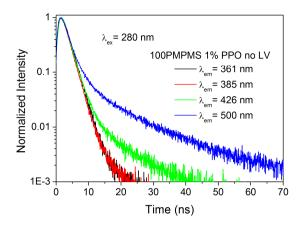
Figure V. 10. Fluorescence decay for a sample with 1% PPO concentration at different wavelengths, excited at 280 nm.
