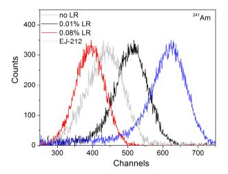
Figure VI. 19. Scintillation spectra produced by α particles for three polysiloxane samples at different LR concentrations, compared to EJ-212.
