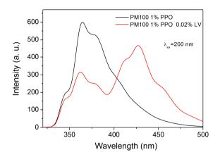
Figure III. 11. Emission spectra of PM100 doped with 1% PPO and with 1% PPO and 0.02% LV, excited at 260 nm.
