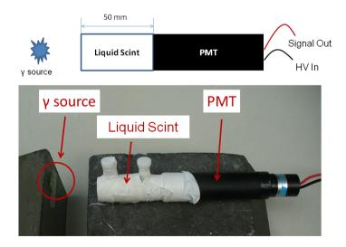
Figure II. 16. Schematic representation and picture of the measurement geometry.
