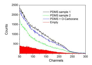
Figure VII. 10. Energy spectra produced by fast neutron on 3D silicon diodes filled with different types of converters.
