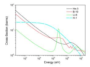
Figure I. 5. Comparison between neutron elastic scattering cross section in hydrogen and the neutron absorption cross section of the most used slow neutron converter in the keV-MeV range.
