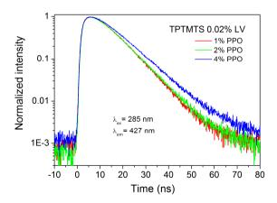
Figure IV. 4. Fluorescence decay spectra for TPTMTS with different concentrations of PPO and 0.02% LV, measured by excitation at 280 nm and emission at 427 nm.
