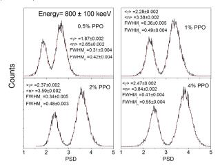
Figure IV. 17. PSD distribution for different TPTMTS solutions with 0.02% LV and variable PPO amount, shown for energy of 800 keVee (keV electron equivalent). Dashed red lines represent the fit used to determine the FoM. Corresponding fitting parameters are also reported.
