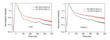
Figure V. 23. Pulse shape comparison between samples with 1% PPO and 8% PPO for neutrons and gamma rays.
