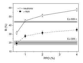
Figure IV. 14. Slow component intensity for neutrons and gamma shapes as a function of PPO concentration.
