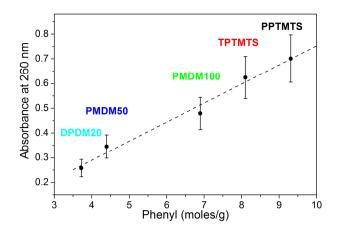
Figure III. 4. Linear correlation between the amplitude of the absorption peak and the amount of phenyl groups in the different polysiloxane liquids.
