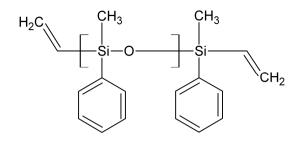
Figure II. 3. Molecular structure of poly(methylphenylsiloxane) vinyl terminated.
