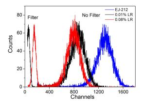
Figure VI. 16. Scintillation spectra, with and without filter, for two samples with 1% PPO, 0.04% LV and two different concentartions of LR (0.01% and 0.08%). EJ-212 is also shown for comparison.
