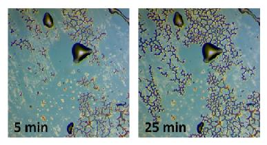
Figure VII. 8. Time evolution of the B<sub>4</sub>C deposit. The increased number of wrinkles is clear.
