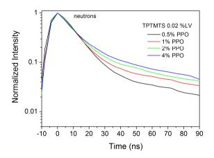
Figure IV. 10. Averaged neutrons scintillation pulse shapes for TPTMTS at different PPO concentrations.
