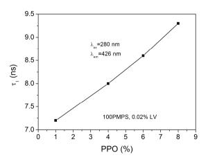
Figure V. 13. Fluorescence lifetime as a function of PPO concentration for polysiloxane scintillators. Emission was recorded at LV emission peak (426 nm) excited at 280 nm.
