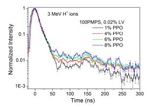
Figure V. 15. 3 MeV proton beam TRIBIL curves at different PPO concentration.
