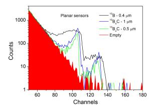
Figure VII. 13. Recorded energy spectra produced by thermal neutrons on planar detectors with different converters.
