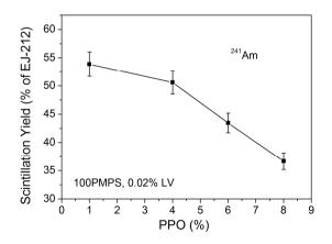
Figure V. 22. Scintillation light yield as function of PPO concentration, measured with <sup>241</sup>Am alpha source.
