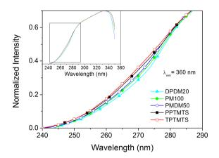
Figure III. 10. Normalized PPO excitation spectrum, measured at 360 nm, for different polysiloxane samples with 1% PPO.
