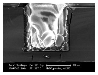
Figure VII. 3. SEM image in cross-section of a silicon cavity filled with polysiloxane.
