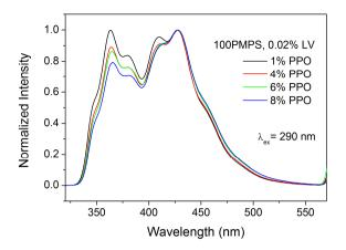
Figure V. 7. Normalized fluorescence emission excited at 290 nm for 100PMPS samples with 0.02% LV and various PPO concentrations.
