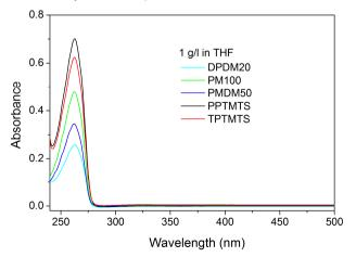
Figure III. 3. Absorption spectra of 1 g/l diluted solutions of different polysiloxane liquids.
