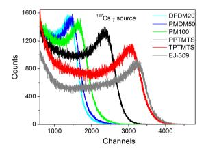
Figure III. 15. Scintillation spectra of polysiloxane based liquid scintillators and EJ-309 measured with <sup>137</sup>Cs γ-source. Spectrum of EJ-309 is also shown for comparison.
