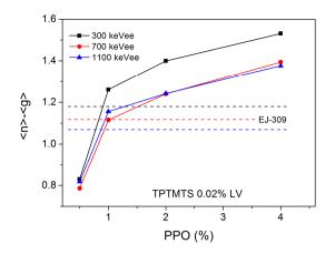
Figure IV. 20. Peak centroids separation as a function of PPO concentration at three different energies. Values for EJ-309 are also shown.
