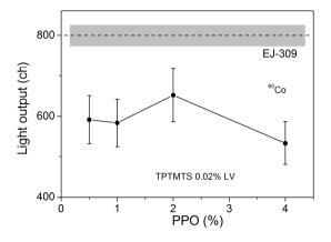
Figure IV. 15. Scintillation light output as a function of PPO concentration with 60Co γ-rays.
