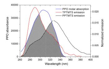
Figure III. 9. PPTMTS and TPMTS emission spectra overlapped to PPO molar absorption. Emission spectra are normalized over the area. Grey areas represent the overlap integral (equation(13)).
