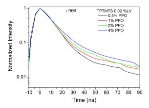
Figure IV. 9. Averaged γ-rays scintillation pulse shapes for TPTMTS at different PPO concentrations.
