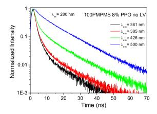
Figure V. 11. Fluorescence decay for a sample with 8% PPO concentration at different wavelengths excited at 280 nm.
