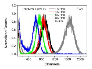
Figure V. 21. Scintillation spectra, measured with <sup>241</sup>Am alpha source at different PPO concentrations. EJ-212 is also shown for comparison.
