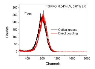
Figure II. 14. Comparison of a 241Am scintillation spectrum collected by a polysiloxane scintillator with or without optical couplant.
