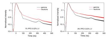
Figure V. 24. Pulse shape comparison between neutron and gamma signals for two different PPO concentrations
