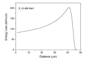
Figure I. 1. Specific energy loss profile along the path for a <sup>241</sup>Am α particle in polysiloxane (spectrum achieved by SRIM simulation [SRIM]).
