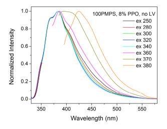
Figure V. 4. Fluorescence emission at different excitation wavelength for a polysiloxane samples with 8% PPO and no LV.
