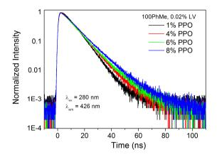
Figure V. 12. Fluorescence lifetime at different PPO concentrations for samples without LV. Excitation wavelength at 280 nm and emission wavelength at 426 nm (LV emission) have been employed for the measurements.
