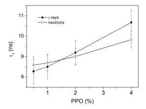
Figure IV. 11. Fast decay time fitting value as a function of PPO concentration in case of neutrons and gamma irradiation.
