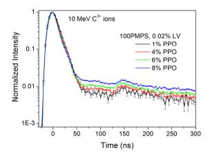
Figure V. 14. 10 MeV C<sup>3+</sup> beam TRIBIL curves at different PPO concentration.
