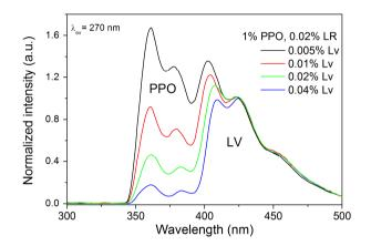
Figure VI. 2. Normalized emission spectra of red emitting polysiloxane samples having 1% PPO, 0.02% LR and different concentrations of LV, excited at 270 nm.
