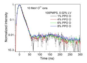
Figure V. 16. 10 MeV O<sup>3+</sup> beam TRIBIL curves at different PPO concentration.
