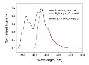
Figure IV. 1. Comparison between emission spectra of TPTMTS with 1% PPO and 0.02% LV, measured with right angle geometry in 10 mm optical path cell and with front face geometry in 2 mm thin optical path cell.
