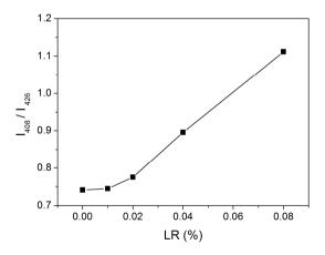
Figure VI. 5. Ratio between the intensity at 408 nm and the intensity at 426 nm as a function of the LR concentration.
