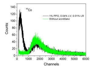
Figure VI. 21. Comparison between the <sup>60</sup>Co gamma spectrum recorded with a red emitting polysiloxane scintillator (0.01% LR) and without scintillator.
