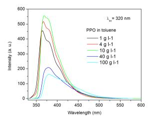
Figure V. 3. Fluorescence emission with excitation at 320 nm different PPO concentrations in toluene.
