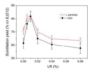
Figure VI. 22. Relative scintillation yield measured by APD for alpha particles and gamma rays as a function of LR concentration.
