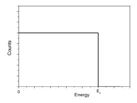
Figure I. 6. Expected energy spectrum of recoil protons produced by scattering on neutrons with energy below 10 MeV on hydrogen atoms.
