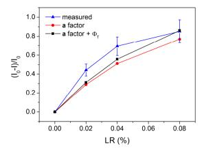
Figure VI. 11. Relative reduction in LV emission intensity as a function of LR concentration. The values are shown as calculated from **a** factor, from **a** factor with addition of non radiative transfer and as measured from fluorescence emission.
