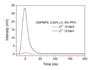
Figure V. 18. Comparison between carbon and oxygen average pulses in a sample with 8% PPO.
