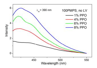
Figure V. 5. Fluorescence emission spectra of different polysiloxane samples, without LV, at different PPO concentrations, excited at 390 nm.
