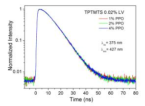
Figure IV. 3. Fluorescence decay spectra for TPTMTS with different concentrations of PPO and 0.02% LV, measured by excitation at 375 nm and emission at 427 nm.
