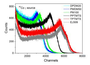
Figure III. 14. Scintillation spectra of polysiloxane based liquid scintillators measured with  $^{60}$ Co  $\gamma$ -source. Spectrum of EJ-309 is also shown for comparison.
