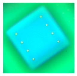
Figure VII. 2. Optical microscope image of the 3D diode, showing the 8 polysilicon columns on the bottom of the cavity.
