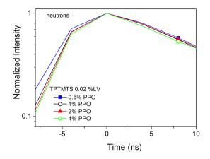
Figure IV. 12. Detail of the neutron induced scintillation pulses, showing the difference in the rise time at the various PPO concentrations.
