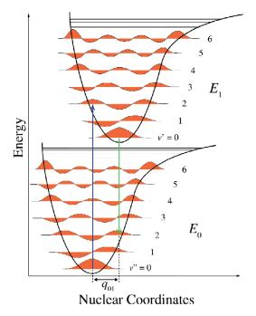
Figure I. 7. Franck-Condon diagram for an electronic transition showing the difference in energy between excitation and de-excitation.
