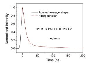
Figure IV. 8. Comparison between measured average pulse shape and fitting function employed to extract the fitting parameters reported in Table IV. 3 and Table IV. 4.
