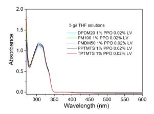
Figure III. 5. Absorption spectrum of polysiloxane liquids doped with 1% PPO and 0.02% LV in 5 g/l THF solutions. PPO absorption peak is visible between 280 nm and 350 nm.
