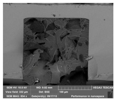
Figure VII. 5. SEM cross-section image of a 3D sensor filled with PDMS containing 30% of metallic <sup>10</sup>B powder.
