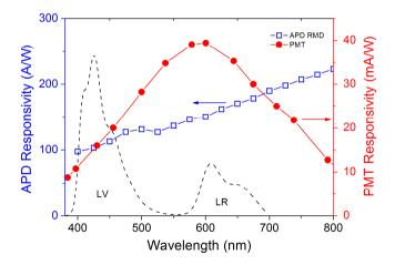
Figure VI. 17. Comparison between the response curve of the red enhanced PMT and APD used in this work. The dashed line shows the typical emission spectrum of red emitting polysiloxane scintillator.
