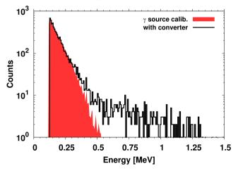
Figure VII. 9. Energy spectrum of fast neutrons compared with that of <sup>60</sup>Co gamma rays, for a sample filled by 22PDPS.
