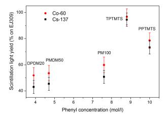
Figure III. 16. Scintillation light yields for different polysiloxane liquid scintillators, relative to EJ-309, as a function of the phenyl concentration.
