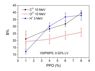
Figure V. 17. Slow decay fractional intensity as a function of PPO concentration measured for carbon ions, oxygen ions and protons.
