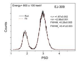
Figure IV. 18. PSD distribution for EJ-309 liquid scintillator, shown for energy of 800 keVee. Dashed red lines represent the fit used to determine the FoM, and the relative fitting parameters.
