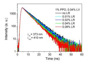
Figure VI. 12. LV fluorescence decays for different LR concentrations.
