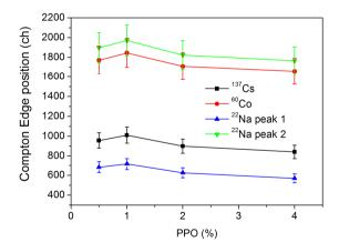
Figure IV. 16. Compton Edge position as a function of PPO concentration evaluated for the different gamma sources.
