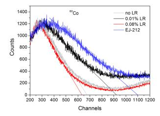
Figure VI. 20. 60Co gamma rays scintillation spectrum, measured by APD for different LR concentrations. Thin lines represent the linear fit used for the determination of the Compton end point.
