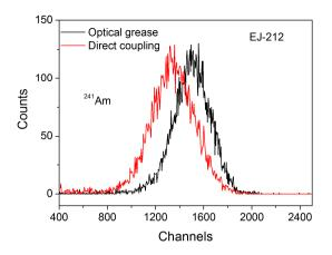
Figure II. 15. Comparison of a <sup>241</sup>Am scintillation spectrum collected by EJ-212 plastic scintillator with or without optical couplant.
