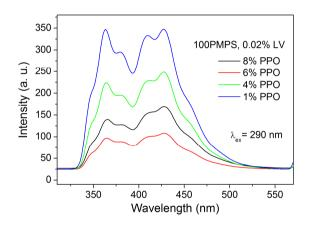
Figure V. 6. As recorded fluorescence emission excited at 290 nm for 100PMPS samples with 0.02% LV and various PPO concentrations.
