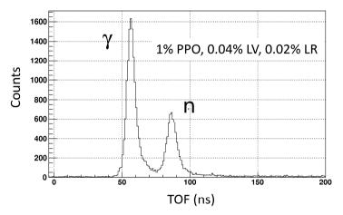
Figure VI. 23. ToF spectrum for a sample with 0.02% LR concentration.
