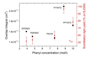
Figure III. 17. Trend comparison between scintillation light yield (from 60Co) and overlap integral for different polysiloxane liquids.
