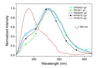
Figure III. 7. Fluorescence emission spectra for different liquid polysiloxane in 1g/I THF solution. Excitation wavelength was fixed at 260 nm for all samples.
