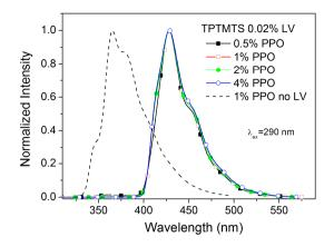
Figure IV. 2. Normalized florescence emission spectra at different PPO concentrations. The emission spectrum of a sample without LV is also shown for comparison.
