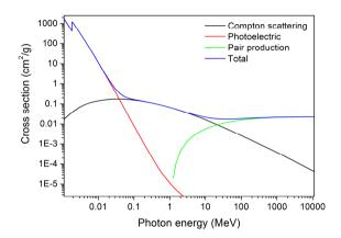
Figure I. 2.γ-rays cross section for the different types of photon interactions as a function of energy in a polysiloxane material (data achieved from [NIST2010]).
