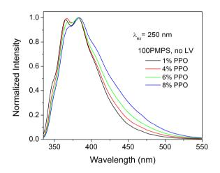
Figure V. 1. Normalized fluorescence emission spectra of polysiloxane samples at different PPO concentrations without LV, recorded with 250 nm excitation.
