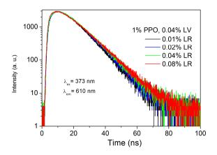
Figure VI. 15. LR emission lifetime at 610 nm with excitation at 373 nm for different LR concentrations
