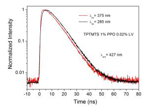
Figure IV. 6. Fluorescence decay for a sample with 1% PPO excited at 280 nm and at 375 nm.
