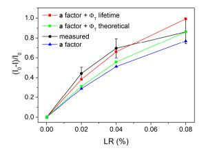
Figure VI. 14. Relative reduction in LV emission intensity as a function of LR concentration. The figure is the same as Figure VI. 11 with the addition of the energy transfer efficiency calculated from the decay times.
