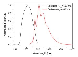
Figure II. 8. Excitation and emission spectrum of the PPO molecule in chloroform.
