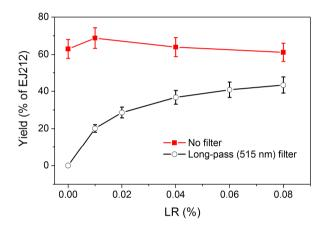
Figure VI. 18. Scintillation light yield, relative to EJ-312, as a function of LR concentration.
