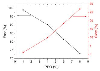
Figure V. 9. Fast and slow component relative intensities, as derived from the fittings of the decay curves, as a function of PPO concentration.
