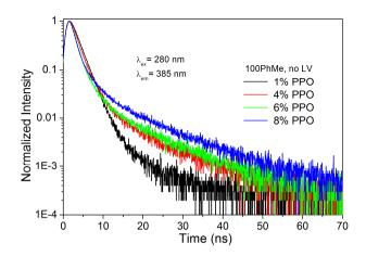
Figure V. 8. Fluorescence lifetime at different PPO concentrations for samples without LV. Excitation wavelength at 280 nm and emission at 385 nm (PPO emission) have been employed for the measurements.
