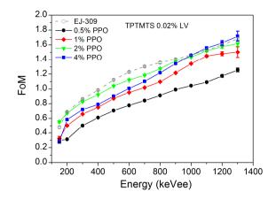
Figure IV. 21. FoM as a function of energy for the different TPTMTS samples and for EJ-309.
