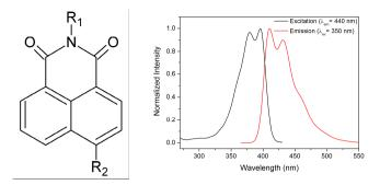
Figure II. 9. (Left) Generic molecular structure of 1,8-Naphthalimide. The substituents R1 and R2 are patented for the LV molecule. (Right) Emission and excitation spectra of the LV molecule in chloroform.
