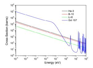
Figure I. 4. Neutron absorption cross-sections for the most used reactions in slow neutron detection [ENDF].
