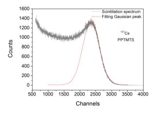
Figure III. 2. Typical <sup>137</sup>Cs scintillation spectrum, with the fitting function used to evaluate the position of the Compton Edge.
