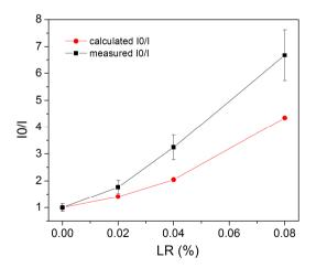
Figure VI. 9. I0/I ratio for different LR concentrations both as measured from fluorescence emission spectra and as calculated from **a** factor.
