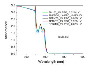
Figure III. 6. Absorption spectrum of undiluted polysiloxane liquids. LV absorption band is visible between 360 nm and 410 nm. Below 350 nm the signal is saturating due to the strong PPO absorption.
