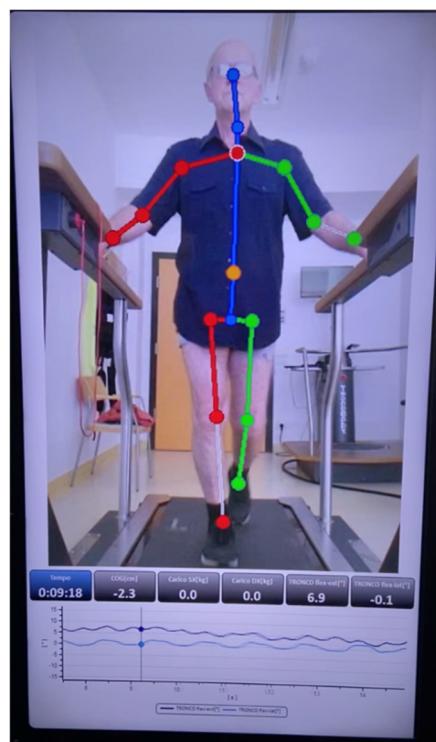
Figure 1. A 69-year-old patient undergoing gait analysis using an instrumented treadmill (WalkerView, TecnoBody MS, Dalmine, Italy). Colored markers represent tracked anatomical landmarks as identified by the system.
