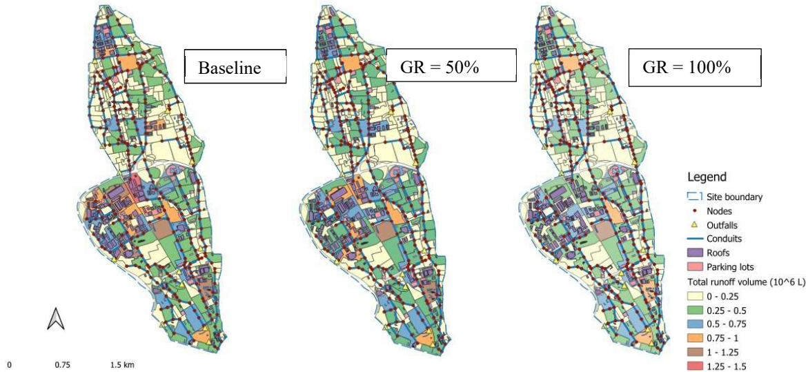
Figure 1. Spatial distribution total runoff volume for each subcatchments
