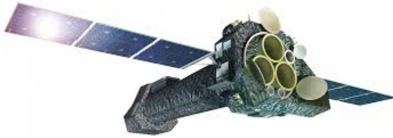
Figure 4.13: The ESA XMM–Newton observatory in flight configuration (optics module, telescope tube, service module, and focal–plane instruments).
