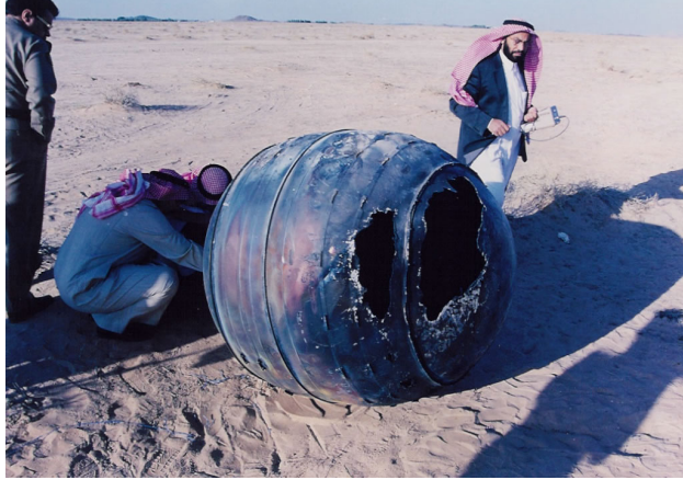
Figure 1.3: Titanium motor casing from a Delta II rocket upper stage that survived atmospheric re-entry and landed in the Saudi Arabian desert in 2001, demonstrating that large debris objects can reach the Earth’s surface after uncontrolled re-entry. Image credit: European Space Agency (ESA).
