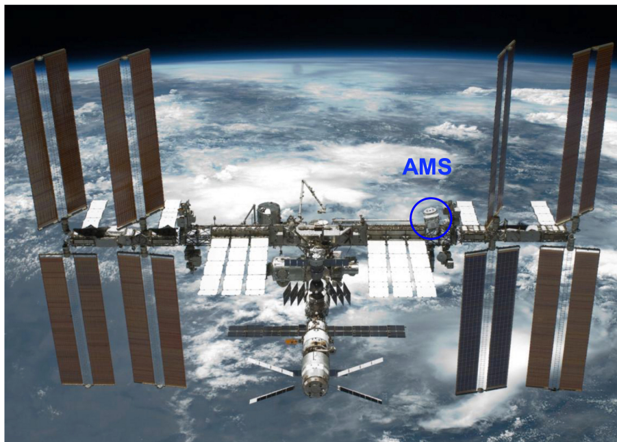
Figure 2.1: AMS is mounted on the ISS with a 12 degree angle to the zenith to prevent the rotating ISS solar arrays from being within the AMS field of view [84].
