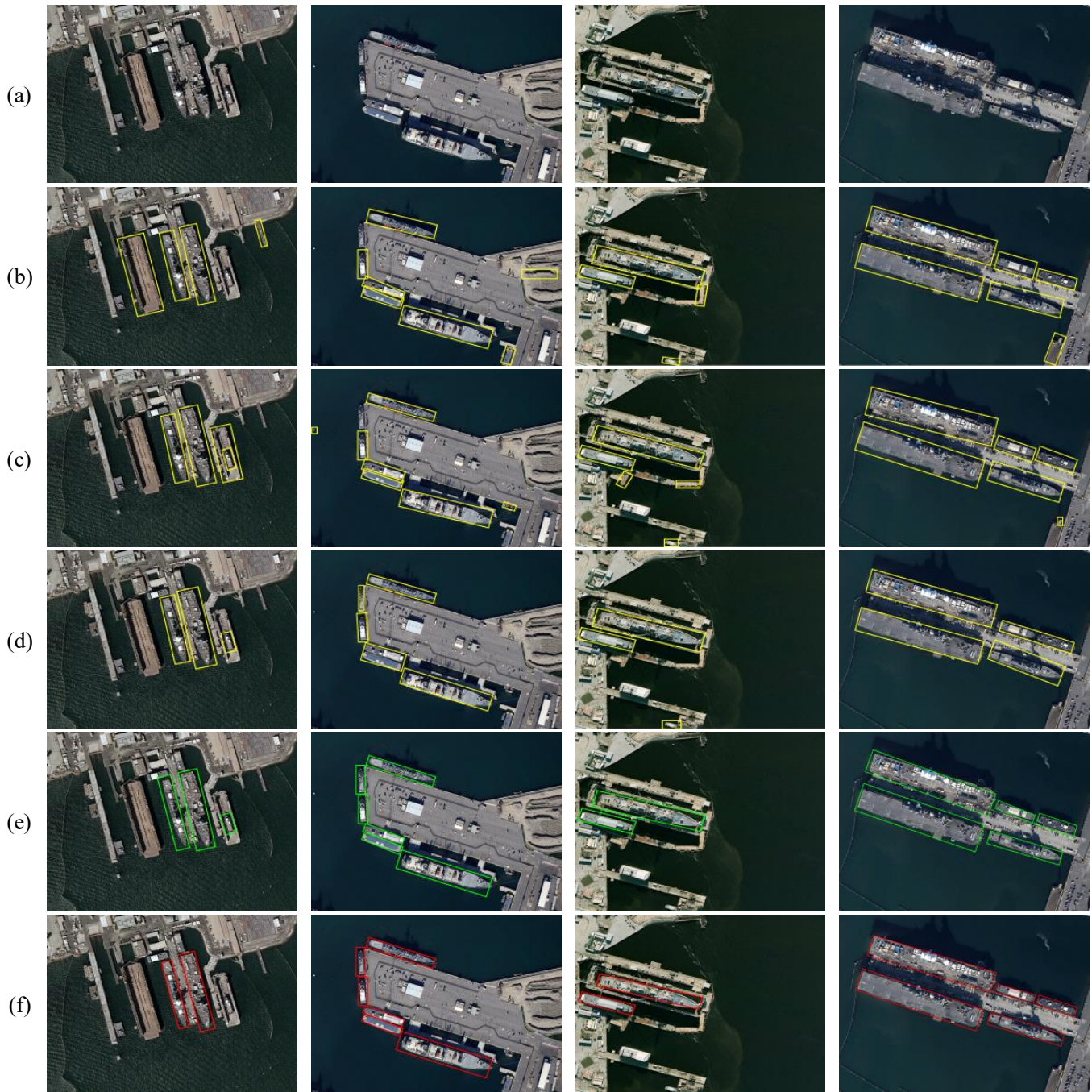
Fig. 7. Examples provided by the different considered methods on the HRSC2016 dataset. (a) Test image, (b) Faster R-CNN, (c) HSF-Net, (d) SSE attention, (e) Proposed method and (f) Ground truth.
