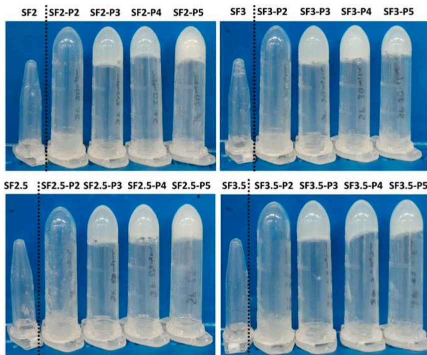
Fig. 3. Inverted vial test for SF-P mixtures: visual assessment of SF-P hydrogelation using different concentrations of SF and P peptide.
