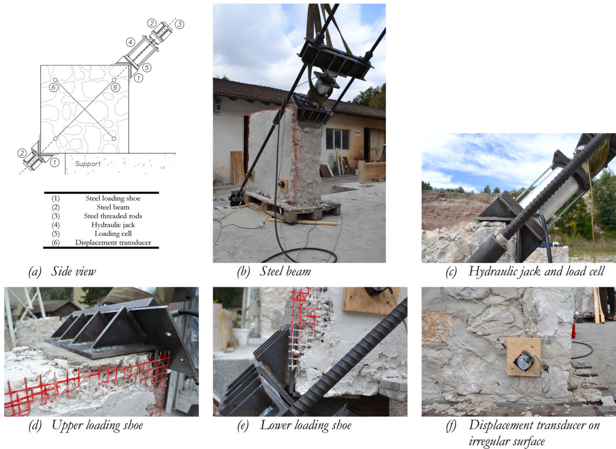
Fig. 5. Test set-up details.
