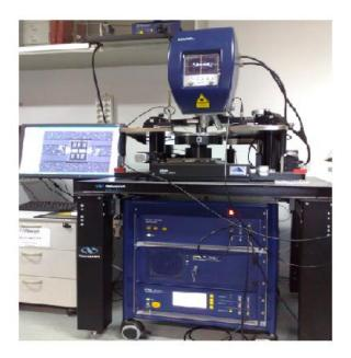
Figure 5.15: Picture of the set up for dynamic measurement.
