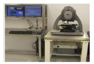
Figure 5.3: The optical 3-D profilometer NewView 6300 from ZYGO.
