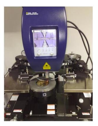
Figure 6.23: Picture of one of the varactors during the transient dynamic characterization.
