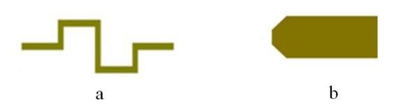
Figure 6.30: Detailed view of the a) meander spring and b) leaf type spring in thin gold.
