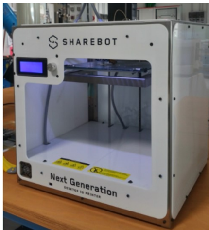
Figure 33. Sharebot NG 3D printer.
