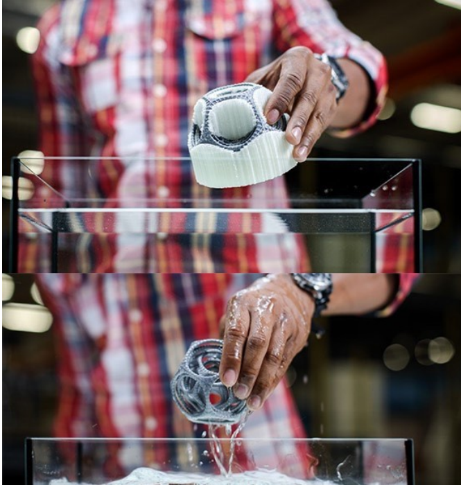
Figure 10. Printing a complex structure with overhanging parts with PVA supports that are then dissolved in water.
