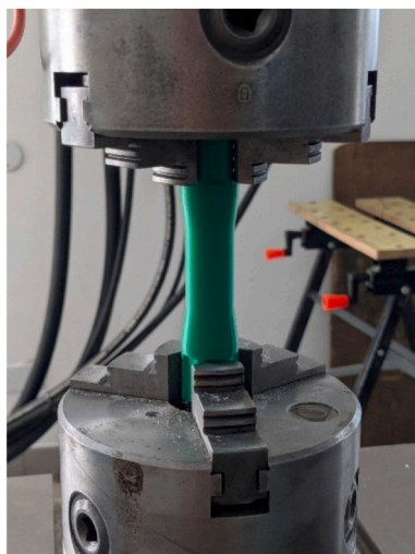
Fig. 5. Biaxial testing machine clamps and an ABS cylindrical specimen.
