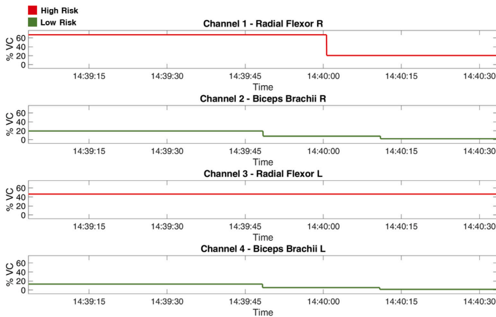
Fig. 15. Muscle-Specific and Time-Oriented % VC: The % VC computed for the four surface electrodes placed on the operator’s upper limbs is depicted for task #3. The values are color-coded based on the EAWS risk level associated with the channel-specific score.
