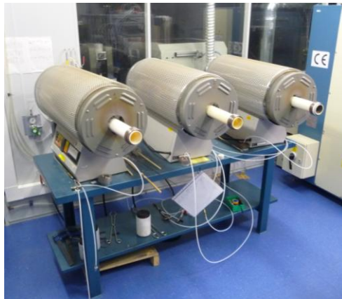
Figure II - 13. Carbolite STF (16/-/610 or STF/-/610) cylindrical furnaces for tubular half-cells cosintering.
