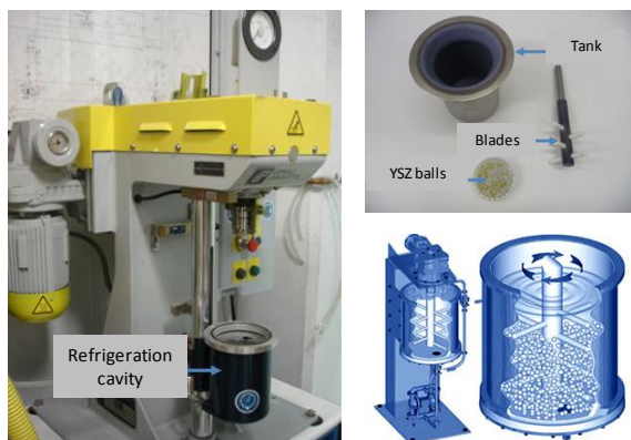
Figure II - 9. 01HD-CE wet grinding attritor.
