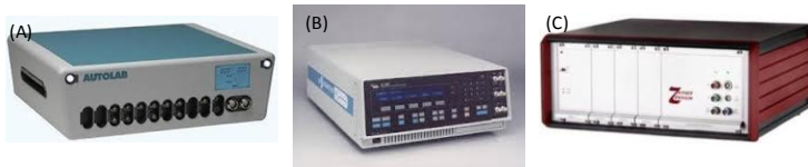
Figure II - 5. Electrochemical Impedance Spectroscopy equipment: (A) Autolab, (B) Solartron and (C) Zanner.
