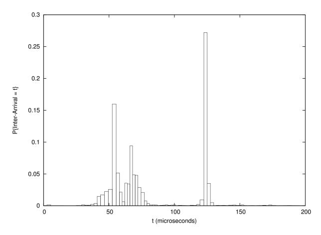
Figure 4: PMF of the inter-arrival times for the network IRQ thread.
