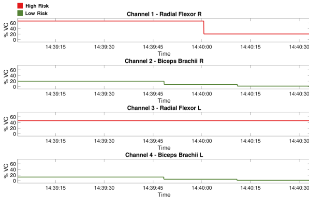
FIGURE 5.15: Muscle-Specific and Time-Oriented % VC: The % VC computed for the four surface electrodes placed on the operator's upper limbs is depicted for task #3. The values are color-coded based on the EAWS risk level associated with the channel-specific score.
