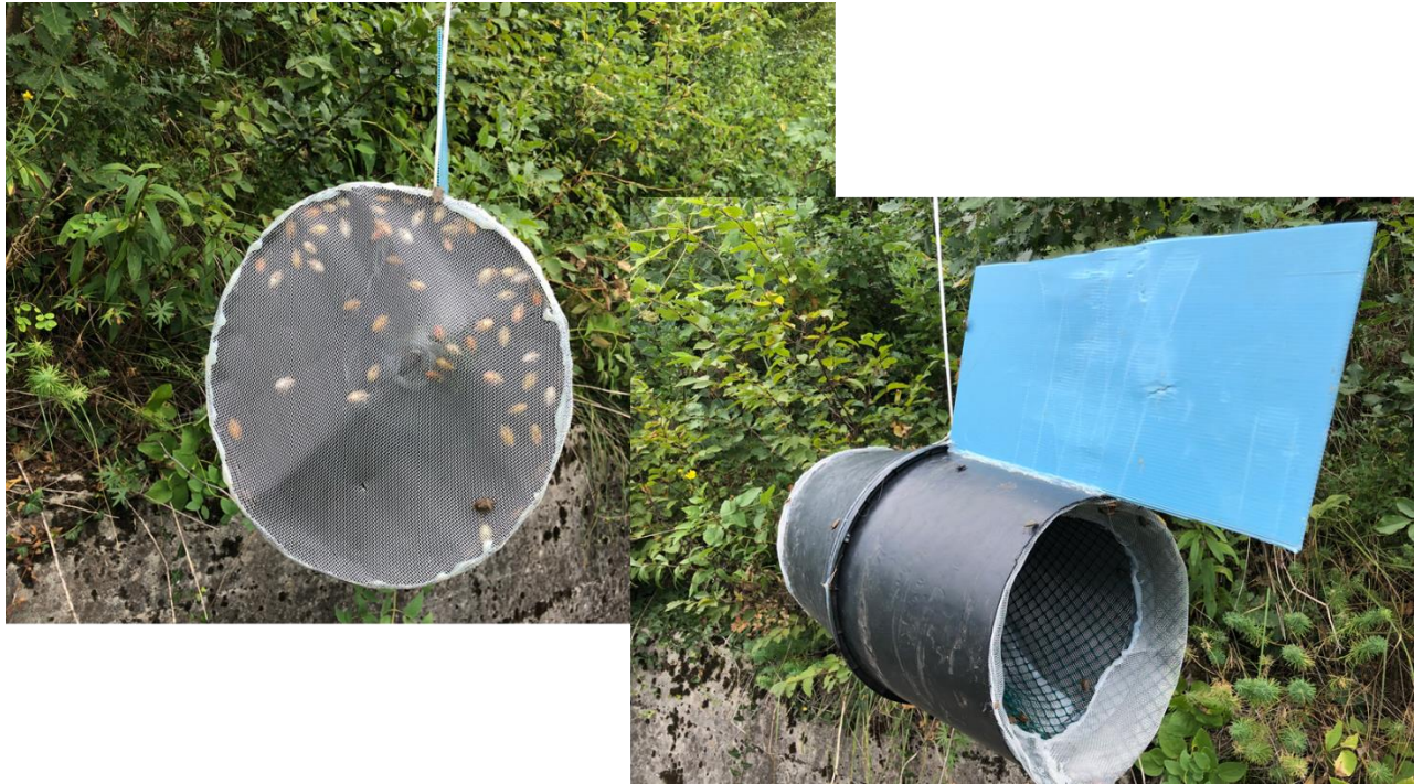
Figure 2.1. Rotating live trap for Halyomorpha halys consisting of two large black flower pots joined in the middle, with bases removed and a removable mesh cone for bug entry and removal, an upwind mesh panel for airflow, and an aggregation pheromone lure, with a wind vane to generate the best plume from the trap.
