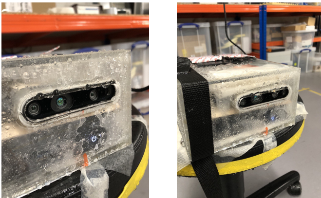
Figure 3.10: The water-resistant enclosure hosting the VO system.
