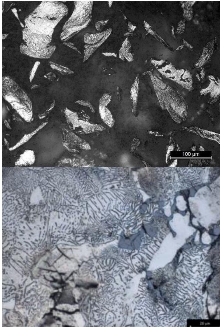
Fig. 5.2 – Microstructure of the AZ91 powder etched with Nital 5% (top) and with HF (bottom).
