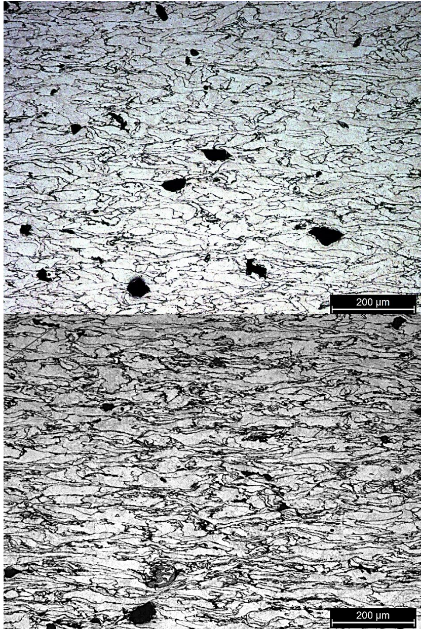
Fig. 5.33 - Pure Mg microstructures after extrusion 330 °C (top) and 380 °C (bottom).
