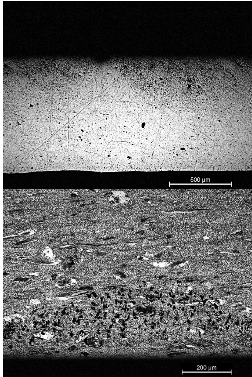
Fig. 5.30 – General view (top) and microstructure evolution on inner region (bottom) of AZ91 tube extrusion.
