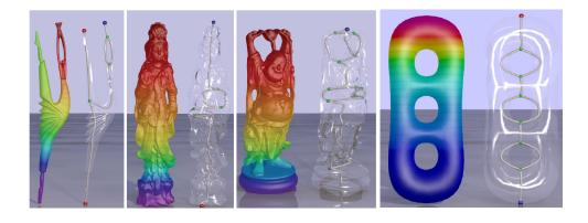
Figure 3.9: The Reeb graphs and their embedding [71]. The colors of the models shows the values of the mapping function. Blue corresponds to the low and red to the high values of the function.
