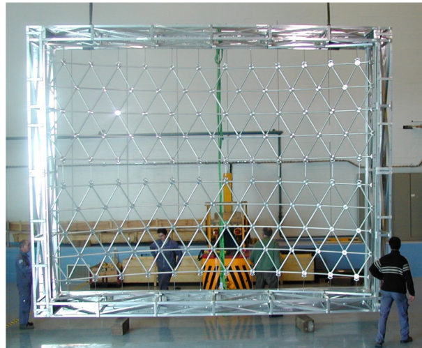
Figure B.14: The mirror support structure; the nodal points are connected by light Al pipes. Picture taken from [131].
