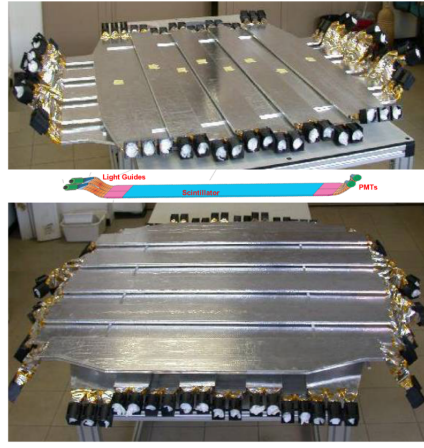
Figure 3.10: Upper and Lower TOF along with a scheme of one of the paddles.
