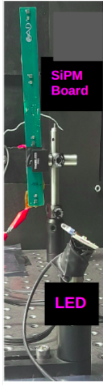
(b) The configuration of the LED and the SiPM bar placed inside the black box.
