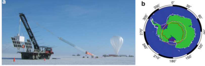
Figure 1.8: a. The CREAM ballooncraft with a 10^6 m^3 balloon at Williams Field near McMurdo, Antarctica. b. The balloon trajectory for a lifetime of 37 days, from December 1, 2008 to January 8, 2010 at the South Pole [2].
