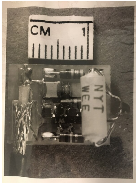
(a) The components of the Kapustinsky LED Pulsar [82].
