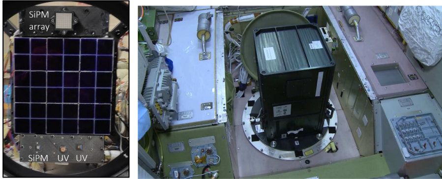
Figure 2.11: The photo-detector module (PDM) is composed of 36 MAPMTs each with 64 independant channels [44] (left) and Mini-EUSO installed inside the the Zvezda module of ISS (right) [50]
