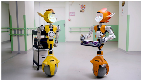
Figure 2.2: The first two prototypes of humanoid ballbot robots developed by Enchanted Tools: Miroki and Miroka.
